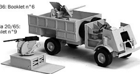
LRDG vehicle inspired by the CMP Ford F-30. The historically correct cargo bed is also provided p. 10. Two variants of a removeable weapons platform are provided.
