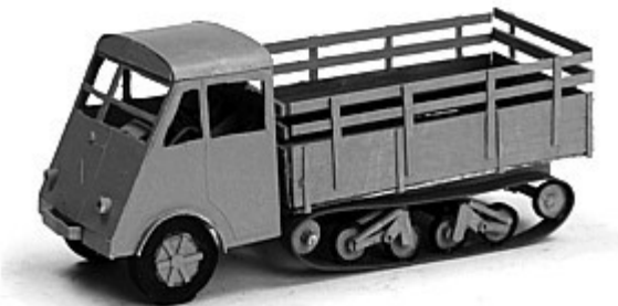
While this " Muletier " (inspired by the Opel Maultier) is fictional, its Horstmann suspension is historically correct.
