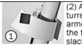
(2) Apply glue to the sides of both the turret top and bottom parts. Glue the armour skirt to them, starting at one of the front edges. Make sure there is no slack on top and on the bottom.
