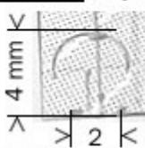
On a piece of rigid paper, draw a semi-circle around the stem of a Q-tip, connect the semi-circle to the 2 mm on the bottom of the piece.
